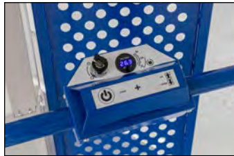
Lockout key & two-hand controls for safety
