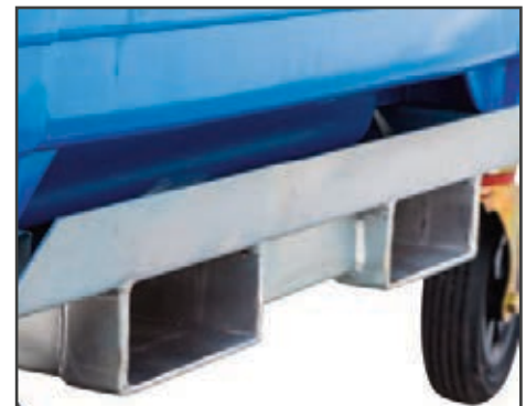
Fork pockets for forklift attachment
